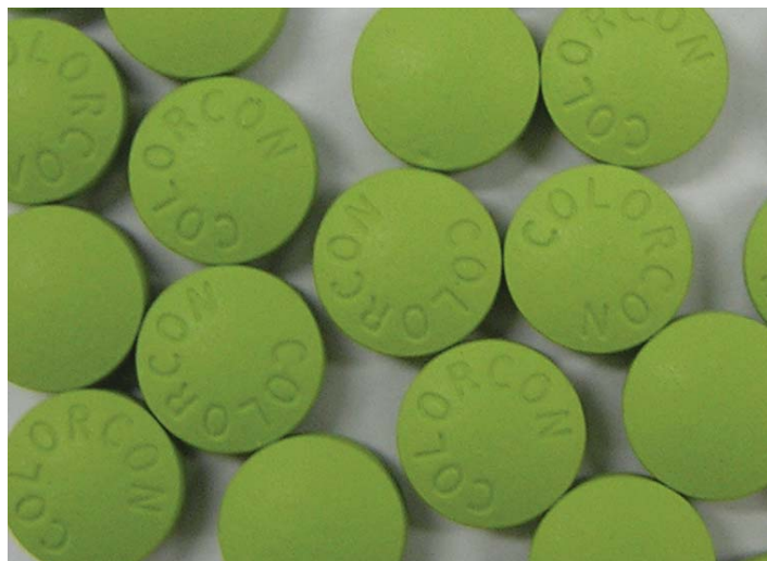
Figure 5 - Picture of XCH Film-Coated Tablets Formula 2 (4% Starch 1500) & Coated with Opadry II 85G 61282 Green
