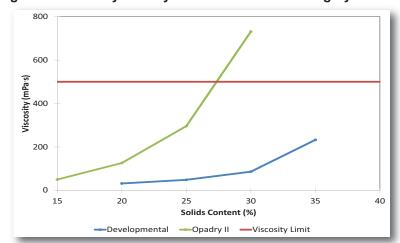
Figure 1. Viscosity of Fully Formulated Film Coating Systems
