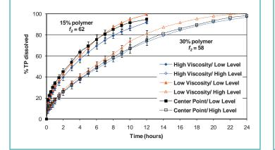
*Figure 2.* Theophylline Release Profiles: Effect of % HP Content (n = 6) (Drug Dissolution Using USP Apparatus II, at 100 rpm with Sinkers and 1000 mL of Deionized Water at  $37 \pm 0.5^{\circ}$ C)
