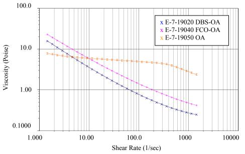
Rheological characterization showed that while the dispersions plasticized with DBS-OA or MCT-OA exhibited shear dependence over a broad range of shear rates the dispersion plasticized with OA showed less of a shear dependence except when approaching shear rates of greater than 1000 sec-1
