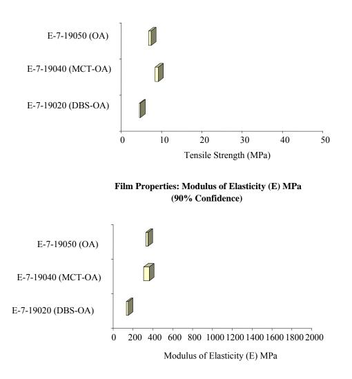
Stress strain plots (above) indicate that while MCT-OA films possessed similar tensile strength to OA films, the MCT-OA films were more ductile in behaviour. However, DBS-OA cast films showed lower overall tensile strength and modulus of elasticity.
