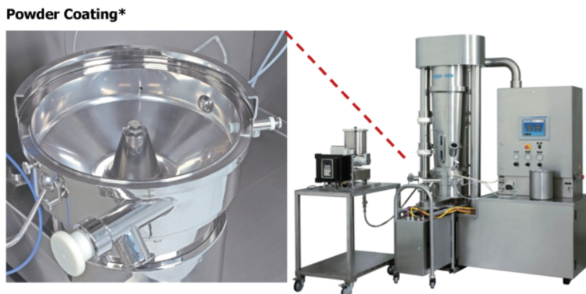
Figure 1. Fluid Bed Equipped with Conical Rotor Insert (Granurex, GXR-35) for Dry Powder Coating*
