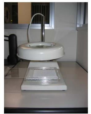
Figure 4. Device for Presenting Tablet Samples for Inspection
