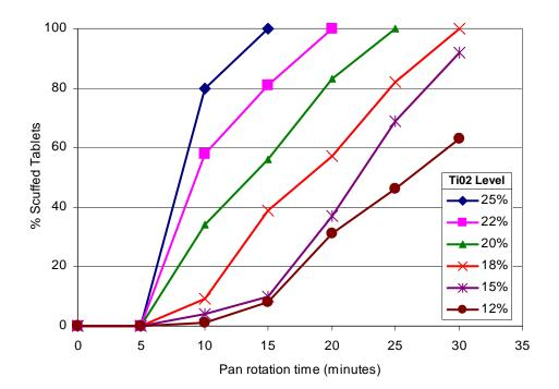
In this test environment, the tablets were simply tumbled and no actual spray was applied to the pre-coated tablets (as opposed to an actual coating environment). These test conditions resulted in much higher levels of scuffing than were observed in subsequent coating trials. The test did, however, demonstrate that adjustments in the level of  $TiO_2$  in the coating formulation can significantly reduce scuffing tendencies.
