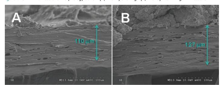
Figure 6. SPM Thickness and Morphology at Low (A, Trial 4) and High (B, Trial 8) Atomizing Air Pressure
