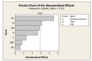
Note: A Pareto chart illustrates the magnitude and the importance of an effect. This chart displays the absolute values of the effects and draws a reference line (2.92), above which a given parameter is considered significant.
