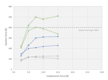
Figure 6: Tablet Ejection Force vs. Compression Force
