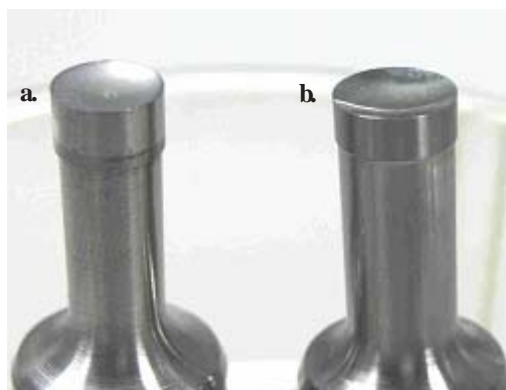
Figure 2 – Punch Tips Condition after Tableting
