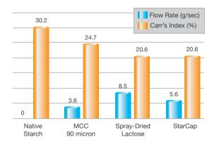
\*Flow rate measured using Sotax FT 300 Flowability Tester, vibration setting 1.7 g
