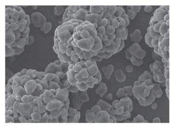
SEM image of StarCap particles
