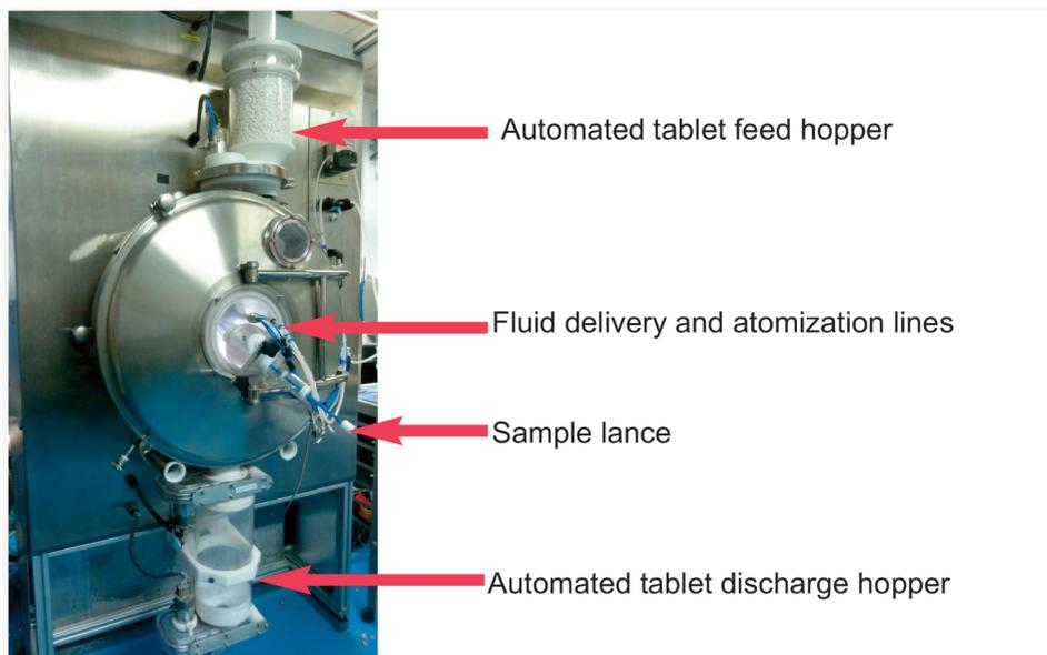
In the ConsiGma Coater, the tablet charge, under the influence of radial air knives, is induced to form a stable cascade inside a perforated drum rotating at high speed (Figure 3).
