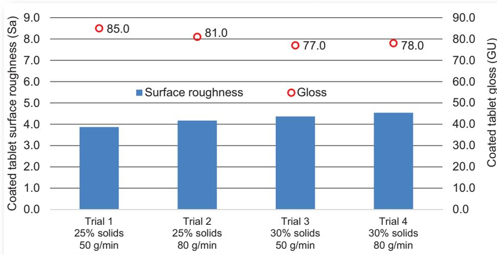
The overall process was very efficient. Coated tablet throughput rates increased from 21 kg/hr to 43 kg/hr as the solids concentration of the coating was increased from 25% to 30% w/w and spray rates increased from 50 g/min to 80 g/min. In the standard twin wheel configuration, this allows throughput rates as high as 86 kg/hour.
