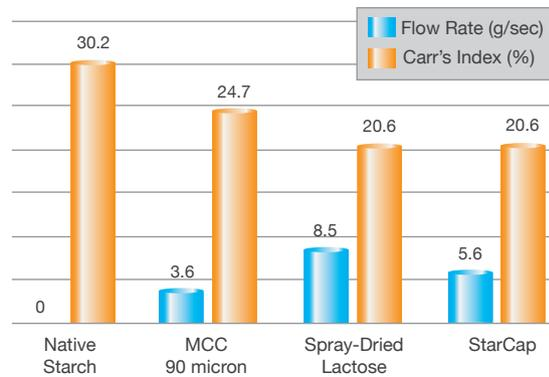
\*Flow rate measured using Sotax FT 300 Flowability Tester, vibration setting 1.7 g
