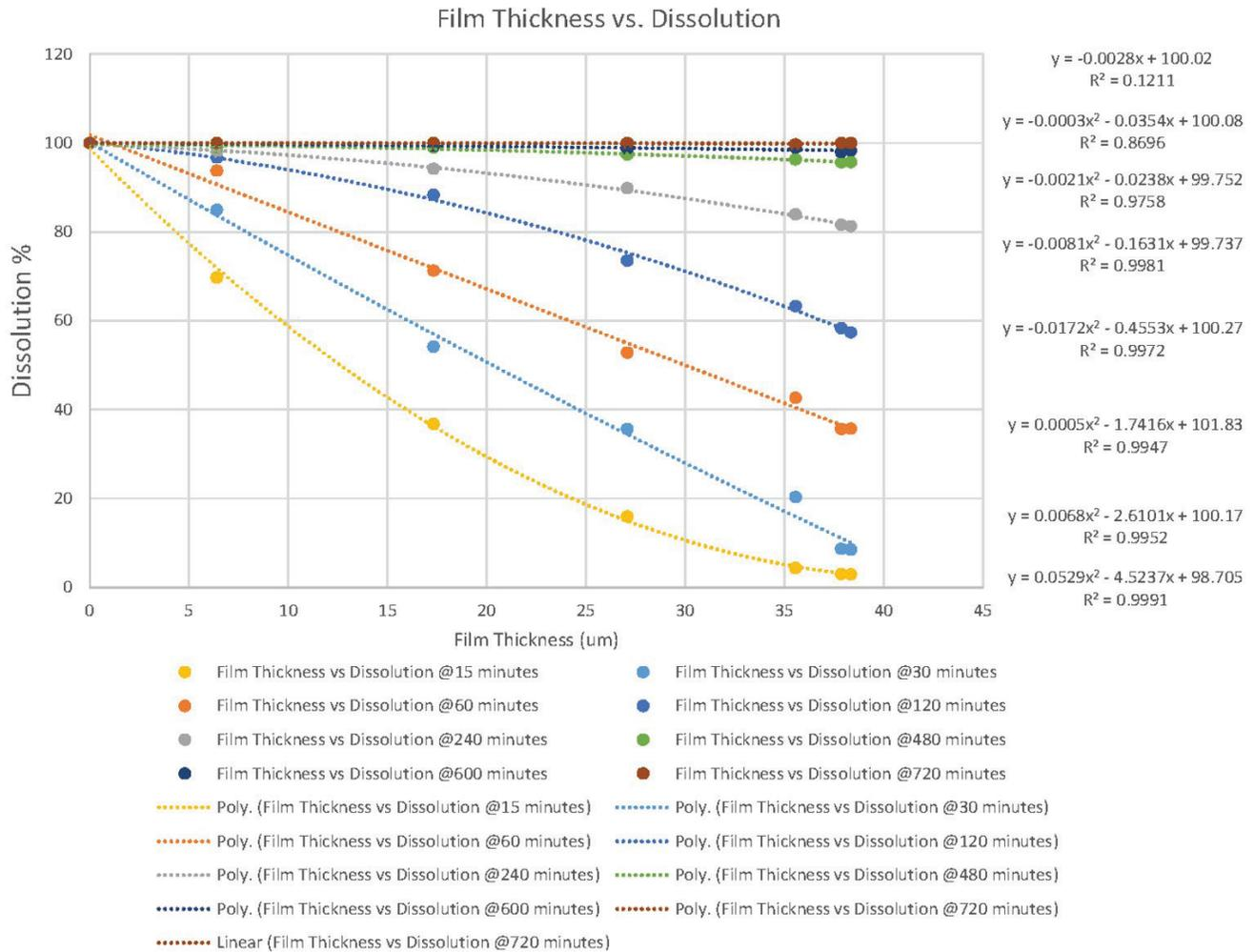
The equations of the best-fit polynomials shown in Figure 6 effectively form the basis of predicting dissolution performance, based on an experimentally determined film thickness. For each given thickness, an equation exists to describe the expected dissolution percentage for each time point measured in CPM-SR-1.
