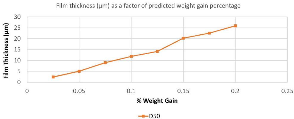
**Figure 5: Film Thickness Measurement of CPM-SR-1 using MDD tool**
