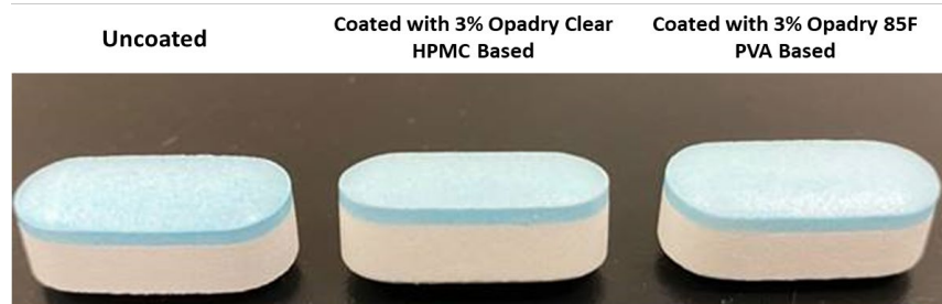
Figure 4. Glipizide IR / Metformin HCl ER FDC Prepared by Rotary Bilayer Tablet Press
