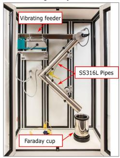
Figure 2c: GranuDrum, Granular Material Flow Analyzer
