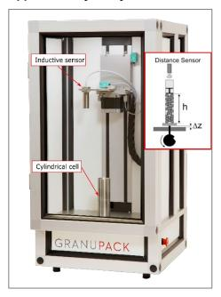
Figure 2b: GranuCharge, Granular Material Electric Charge Analyzer
