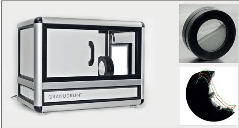
Figure 2c: GranuDrum, Granular Material Flow Analyzer
