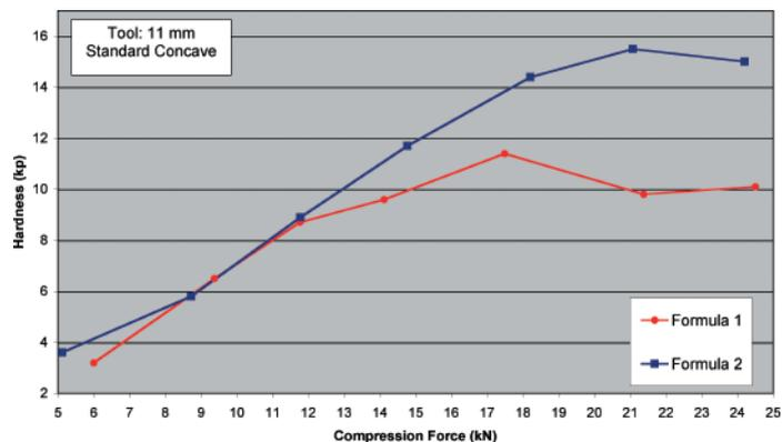
Figure 1: Tablet hardness
