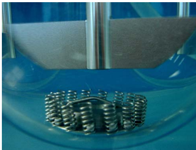
Figure 3. Use of a Novel Sinkers for Dissolution Testing of Enteric-Coated Mini-Tabs
