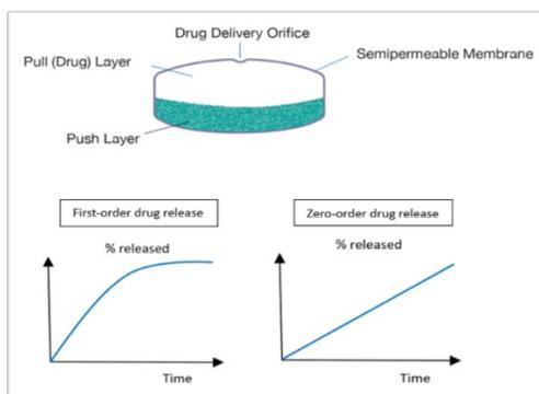
Tablets were coated with Opadry® CA fully formulated osmotic coating system to a 10% weight gain and then laser drilled to create a 0.5 mm delivery orifice on the drug layer tablet face. Glipizide PPOP release profiles were measured in simulated intestinal fluid pH 7.5 over the course of 24 hours.
