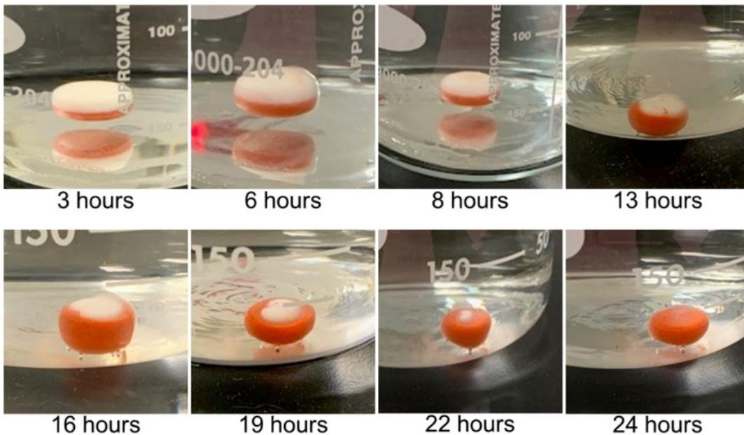
**Figure 5. Drug Release Profiles for Glipizide 11.2 mg PPOP Tablets; Opadry CA Coating at 10 % WG**
