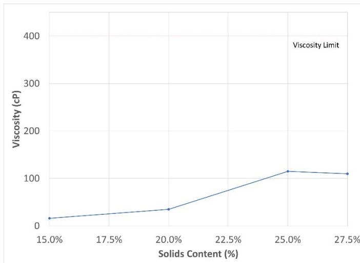
The low viscosity at high solids (27.5%) allows for coating times to be reduced by 45% in compared to 15% solids and a 27% reduction compared to 20% solids, see Figure 3.
