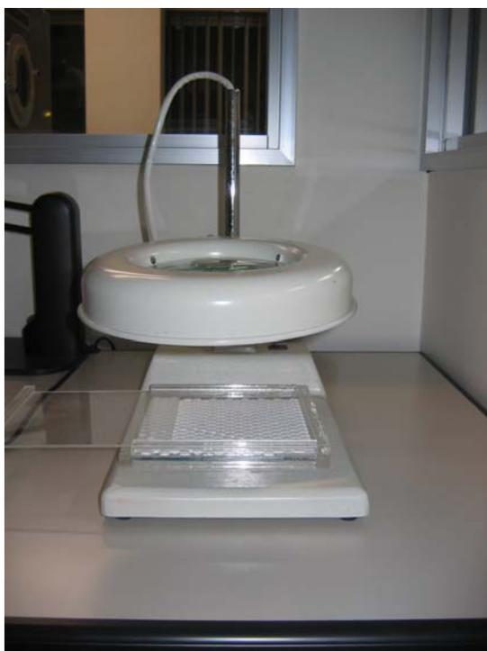
**Figure 4. Device for Presenting Tablet Samples for Inspection**
