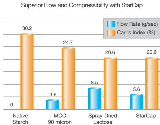
\*Flow rate measured using Sotax FT 300 Flowability Tester, vibration setting 1.7 g
