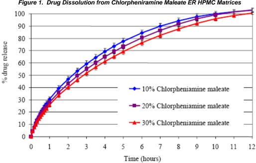
Figure 1. Drug Dissolution from Chlorpheniramine Maleate ER HPMC Matrices
