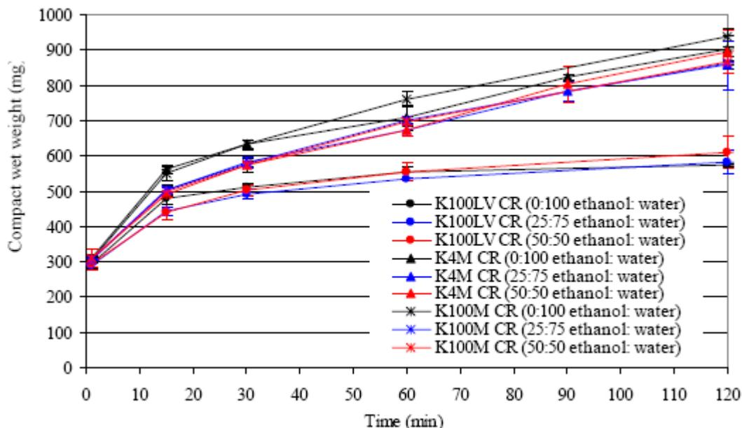
The effect of 1 hour exposure to hydro-alcoholic media on HPMC matrices containing metformin HCl is presented in Figure 2. Any differences in drug release profiles can be explained by a decrease in the saturated drug solubility from 450 g/L (in water) to 379 (in 5% v/v ethanol) and to 295 g/L (in 40% v/v ethanol).
