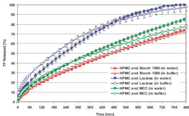
**Figure 4.** Theophylline release from HPMC matrices containing different fillers manufactured at 14 kN in water and phosphate buffer (pH 7.4). [Color figure can be seen in the online version of this article, available on the website, [www.interscience.wiley.com](http://www.interscience.wiley.com).]
