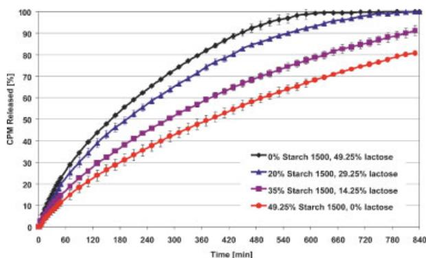
**Figure 5.** Effect of Starch 1500 levels on chlorpheniramine mleate release from HPMC matrices manufactured at 14 kN. [Color figure can be seen in the online version of this article, available on the website, [www.interscience.wiley.com](http://www.interscience.wiley.com).]
