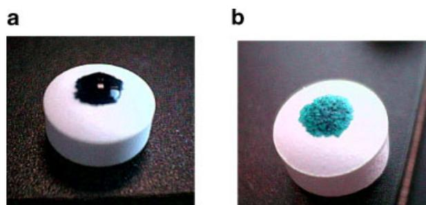
**Figure 7.** Water droplet and its absorption into (a) PPS and (b) microcrystalline cellulose or lactose containing HPMC matrices. [Color figure can be seen in the online version of this article, available on the website, [www.interscience.wiley.com](http://www.interscience.wiley.com).]
