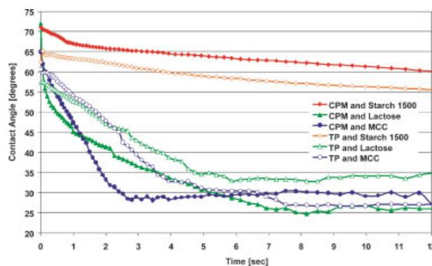
**Figure 8.** Contact angle measurements for water droplets on the surface of HPMC matrices containing different fillers. [Color figure can be seen in the online version of this article, available on the website, [www.interscience.wiley.com](http://www.interscience.wiley.com).]
