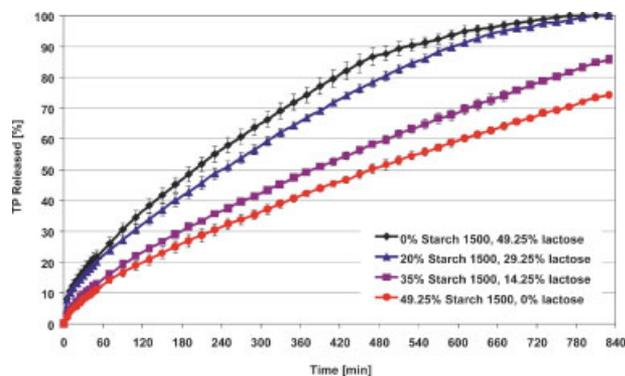
**Figure 6.** Effect of Starch 1500 levels on theophylline release from HPMC matrices manufactured at 14 kN. [Color figure can be seen in the online version of this article, available on the website, [www.interscience.wiley.com](http://www.interscience.wiley.com).]
