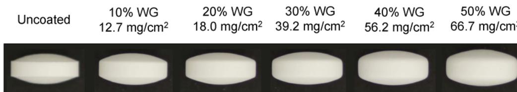
The bulk and pigmented coating provided a high surface gloss as shown in Figure 2. The application of the clear top-coat provided an exceptionally high gloss finish of 138 GU, with a very elegant final appearance.
