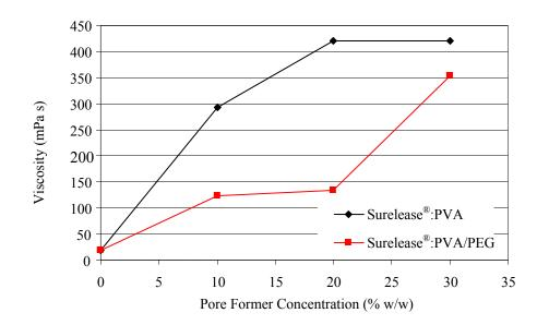
Figure 1. Viscosity Profiles of Surelease<sup>®</sup> Dispersion (15% solids) Containing PVA or PVA/PEG
