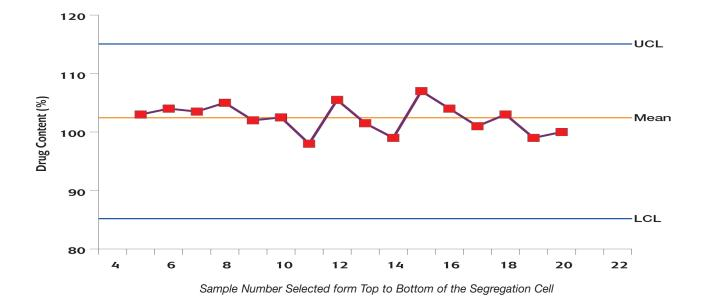
Figure 4: Segregation Profile for the Formulation Prepared with Starch 1500 as a Carrier for the Active-Premix (RSD = 3%)
