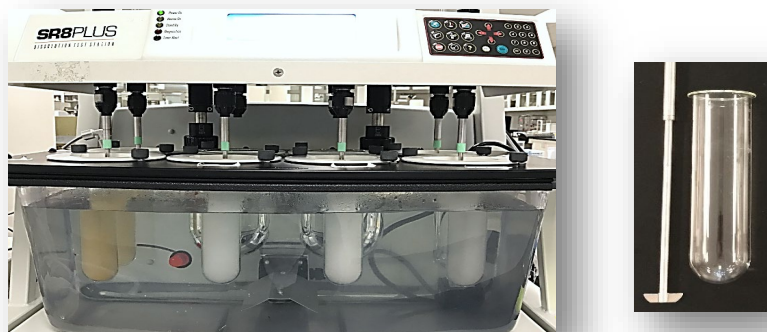
Figure 1. Small Volume Dissolution Set Up For High Throughput Screening
