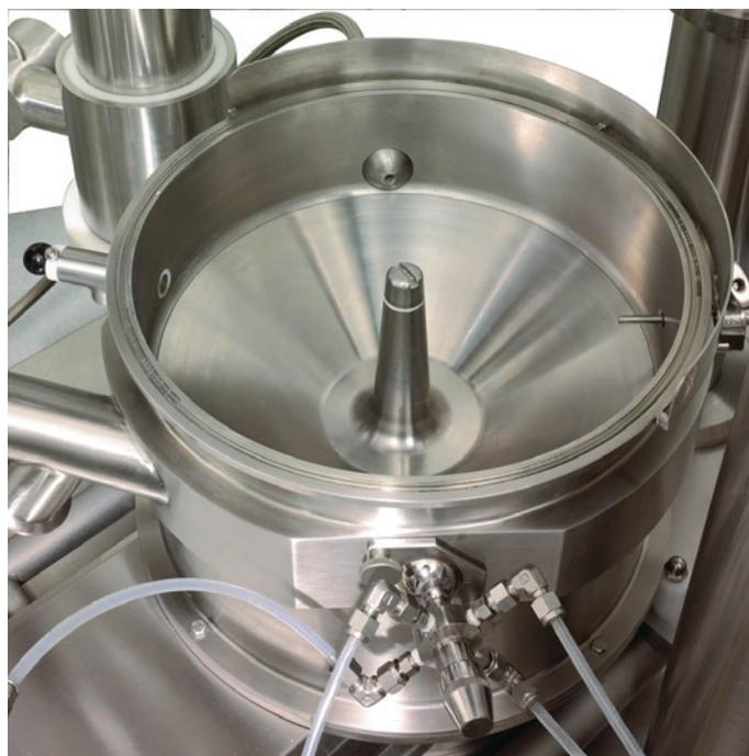
Figure 2. GRANUREX® GXR-35 Rotor.
