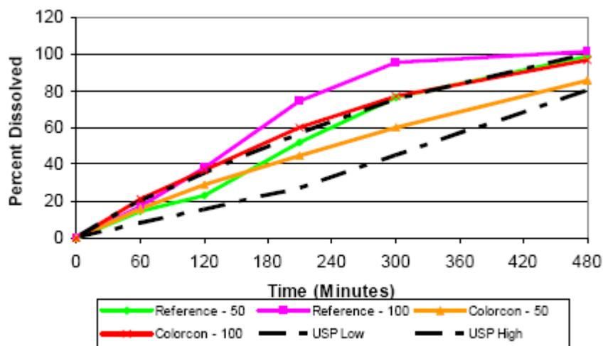
Both formulations showed a faster release at higher level of agitation and sensitivity to hydrodynamic conditions. It has been reported that improper formulation techniques such as low levels of the matrix forming polymer can lead to failure of the dosage form with complete, rapid release of the drug in vivo.<sup>4</sup>
