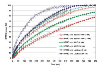
**Figure 1.** The influence of compression force (4 and 14 kN) on chlorpheniramine maleate release in water from HPMC matrices containing different fillers. [Color figure can be seen in the online version of this article, available on the website, www.interscience.wiley.com.]
