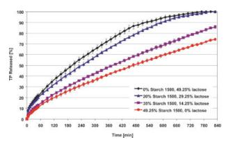
**Figure 6.** Effect of Starch 1500 levels on theophylline release from HPMC matrices manufactured at 14 kN. [Color figure can be seen in the online version of this article, available on the website, www.interscience. wiley.com.]
