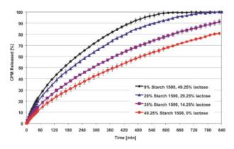
**Figure 5.** Effect of Starch 1500 levels on chlorpheniramine mleate release from HPMC matrices manufactured at 14 kN. [Color figure can be seen in the online version of this article, available on the website, www. interscience.wiley.com.]
