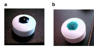
**Figure 7.** Water droplet and its absorption into (a) PPS and (b) microcrystalline cellulose or lactose containing HPMC matrices. [Color figure can be seen in the online version of this article, available on the website, www.interscience.wiley.com.]
