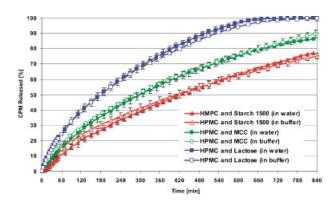
**Figure 3.** Chlorpheniramine maleate release from HPMC matrices containing different fillers manufactured at 14 kN in water and in phosphate buffer (pH 7.4). [Color figure can be seen in the online version of this article, available on the website, www.interscience. wiley.com.]
