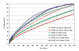
**Figure 2.** The influence of compression force (4 and 14 kN) on theophylline release in water from HPMC matrices containing different fillers. [Color figure can be seen in the online version of this article, available on the website, www.interscience.wiley.com.]
