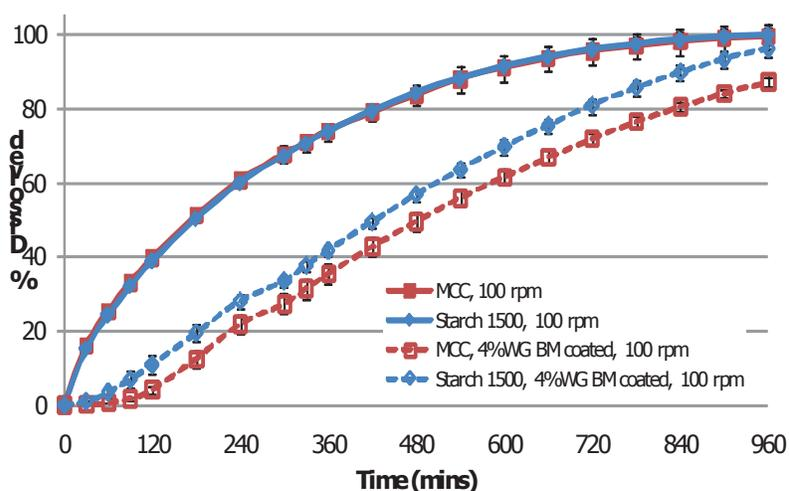
Application of BM coating at 4% WG resulted in elimination of burst release with a lag phase in drug release profile. Near zero order release was obtained for both fillers with  $f_2=56$  at 100 rpm. This was achieved through rupture of BM coating around the belly band area of the matrix tablets, while the ruptured coating remained intact on tablet surfaces. Increasing the coating weight gain resulted in reduction of drug release rate from BM coated matrices.
