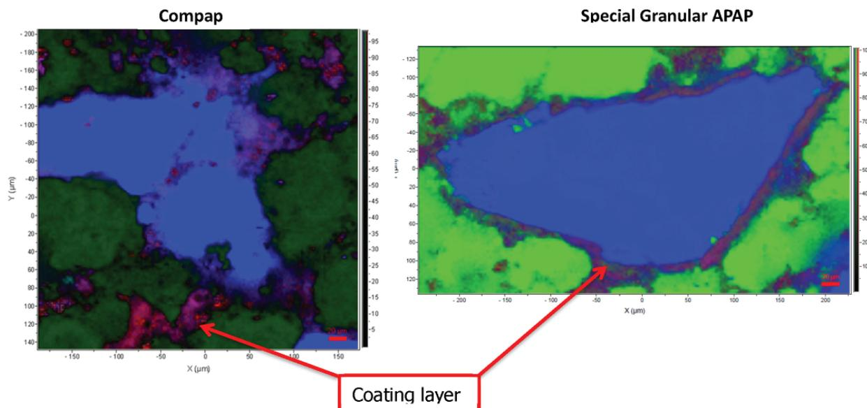
Further individual component spectral analysis was carried out by retaining the coating layer (Surelease) component spectra (purple) and eliminating all other component spectra from the analysis. This highlighted the differences in coating layer integrity between the particles of different morphology (Figure 4).
