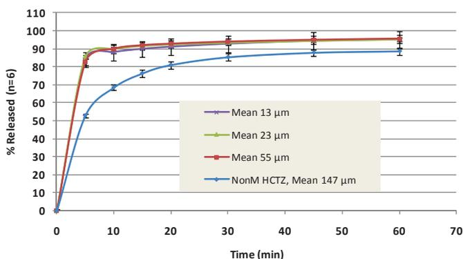
Figure 4. Comparative Dissolution Profiles of 10% HCTZ Tablets Containing 1:2 Ratio of Starch 1500/MCC (n=6)
