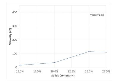
The low viscosity at high solids (27.5%) allows for coating times to be reduced by 45% in compared to 15% solids and a 27% reduction compared to 20% solids, see Figure 3.
