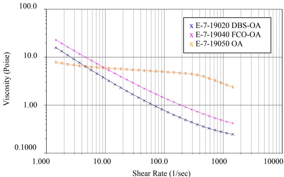
Rheological characterization showed that while the dispersions plasticized with DBS-OA or MCT-OA exhibited shear dependence over a broad range of shear rates the dispersion plasticized with OA showed less of a shear dependence except when approaching shear rates of greater than 1000 sec<sup>-1</sup>
