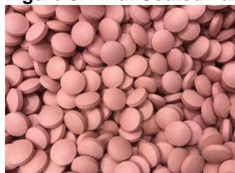
The process resulted in a tablet coating throughput rate of 26.4 kg/h. Coated tablets, sampled from each chamber at the end of the trial, were smooth, uniform in color and free of visual defects (Figure 3).
