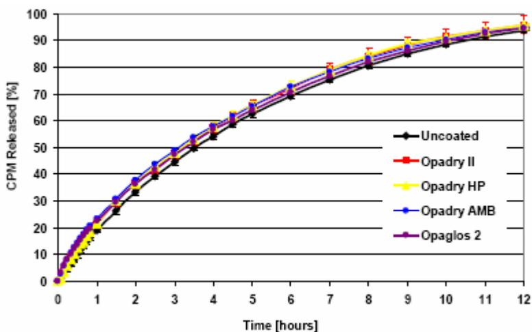
**Figure 3. CPM Release after 12 months Storage at 40°C/75%RH**
