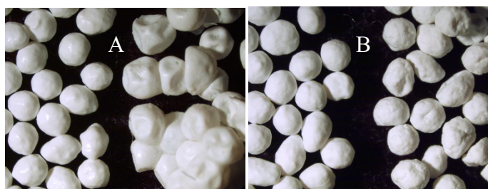
Figure 4: Optical Microscope Images of Pellets before (MPs on the Left) and After Exposure to pH 4.5 (MPs on the Right): (A) without Fumed Silica; (B) with 1.0% Fumed Silica Sprayed.
