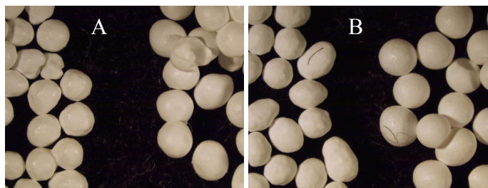
Figure 4: Optical Microscope Images of Pellets before (MPs on the Left) and After Exposure to pH 4.5 (MPs on the Right): (A) without Fumed Silica; (B) with 1.0% Fumed Silica Sprayed.
