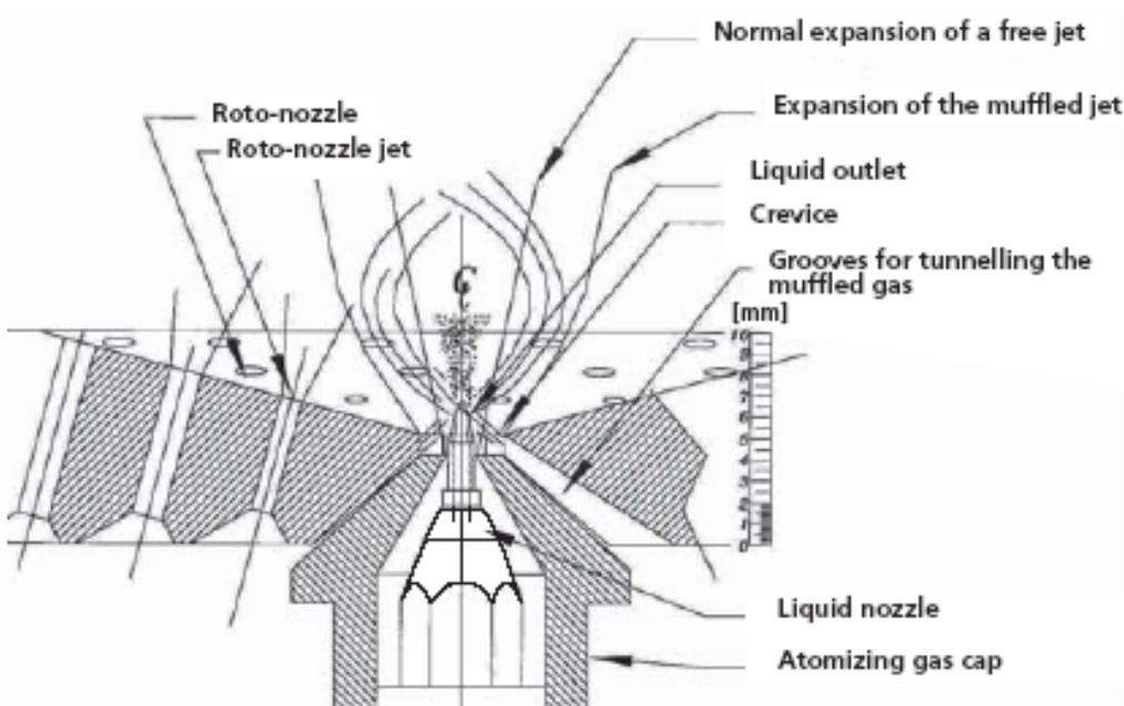
The atomizing air is mixed with low-pressure drying air to dissipate the momentum generated in the atomizing process and reduce the potential for edge attrition of the tablets when striking the coater surfaces.<sup>2</sup> After coating, the tablets or capsules are pneumatically conveyed out of the coating chamber.
