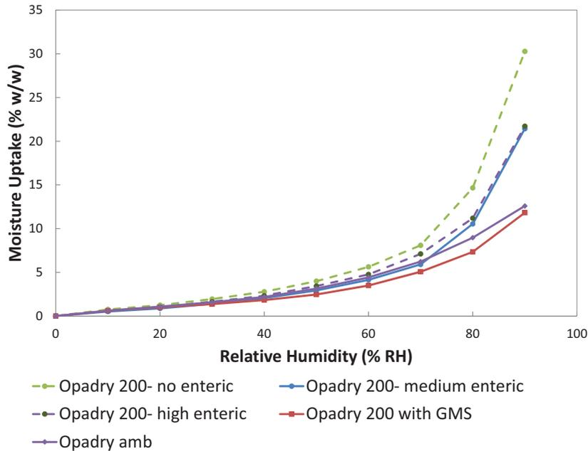
The WVTR values and moisture uptake levels of the coating formulations at 25°C and 80% RH are compared in Figure 4. In general it can be seen that lower moisture uptake values are associated with lower WVTR values. This is likely due to the fact that higher moisture uptake levels will lead to larger moisture concentration gradients through the film thickness and accelerate moisture transmission rates.<sup>4</sup>
