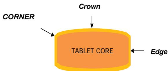
**Figure 2. Schematic Diagram Showing the Top-View of a Tablet.**
