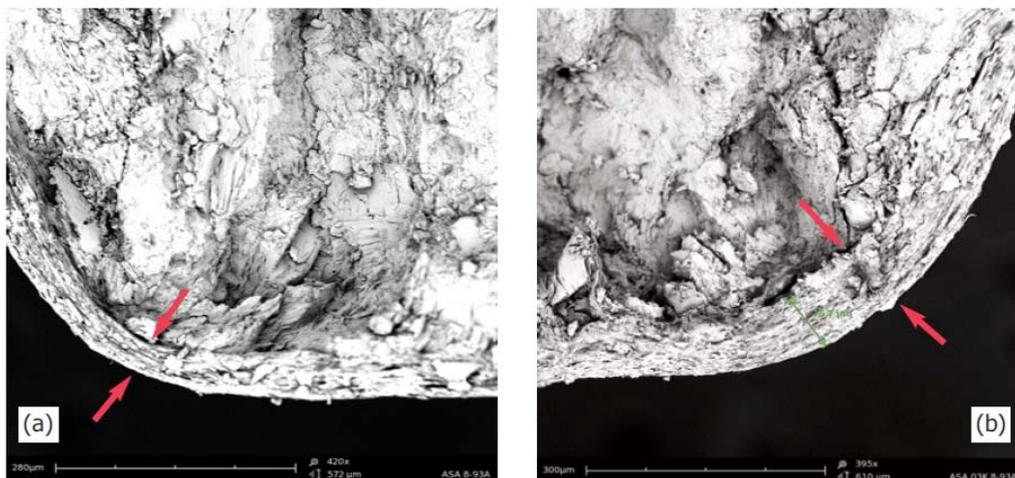
Figure 6 shows the film thickness as a function of coating weight gain for both 6 and 10 mm tablets. The coating thickness on the crown of the tablet was consistently greater than that on the corners or edges of the tablets. SEM was unable to distinguish the clear Opadry seal-coat from the Acryl-EZE functional coating, and, therefore, the thickness of the seal-coated samples represents total film coating thickness. At lower levels of coating weight gain, film thicknesses were
