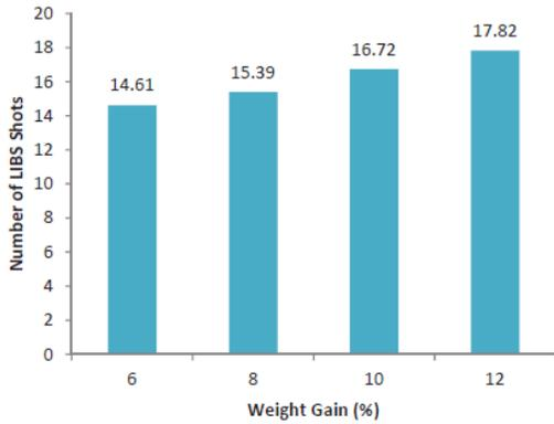
**Figure 12. Plot of Relative Enteric Film Thickness, or Depth, as Measured by LIBS Vs. the Amount of Coating Applied Per Unit Surface Area.**
