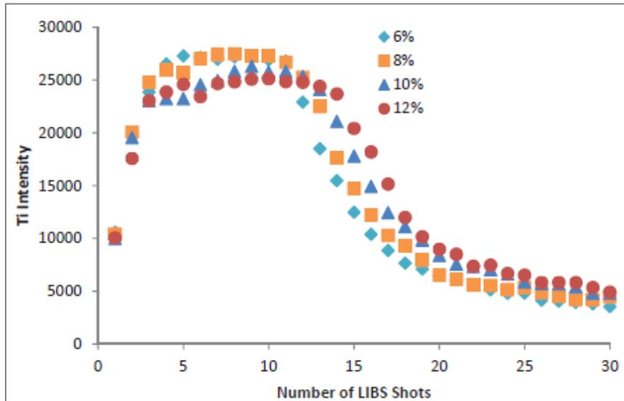
By determining the number of laser shots required to reach  $\frac{1}{2}$  signal maximum and comparing those values vs. the theoretical weight gains, we constructed **Figure 11**. This figure shows that with increasing weight gain, a higher number of laser shots were required to penetrate through the entire enteric film coating.
