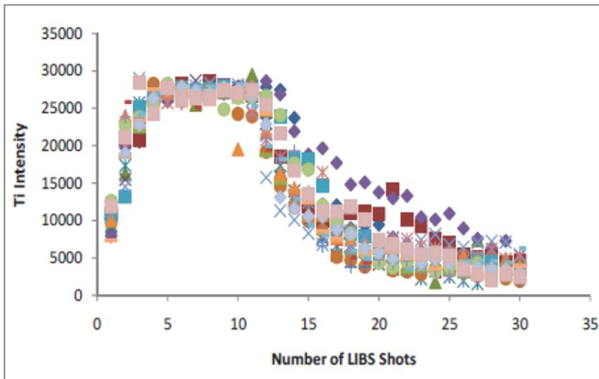
**Figure 9. Titanium Signal Intensity for 6% Weight Gain on 6 mm Core without Sub-coat.**
