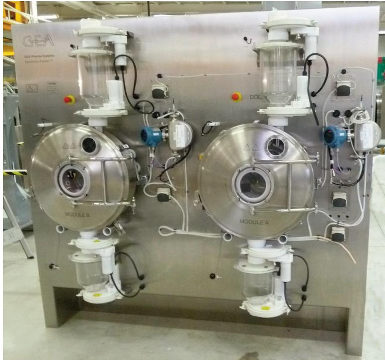
In this study, tablets were automatically fed into a single coating module with automated discharge at the completion of each coating cycle in a semi-continuous process. The single coating chamber configuration is shown in Figure 3.
