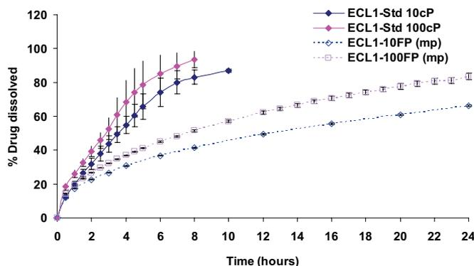
**Figure 4. Dissolution Profiles of Theophylline Tablets (ECM1) (TP/ EC / MCC = 1:1:1, Compression Force: 10 kN)**
